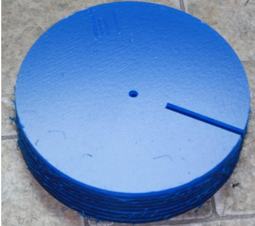
Now pull off the protective (blue) layer from both surfaces of the disc.
