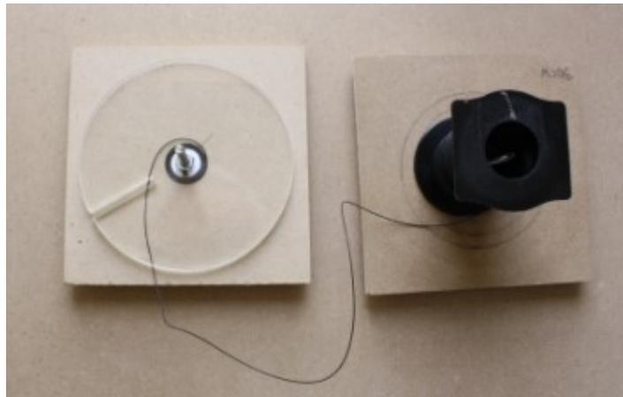
Now we will need to use a 2" ABS Pipe Cap to hold the disc down during winding. Otherwise the winding will rise and we will get doubled turns. The cap is just a temporary aid during winding.
