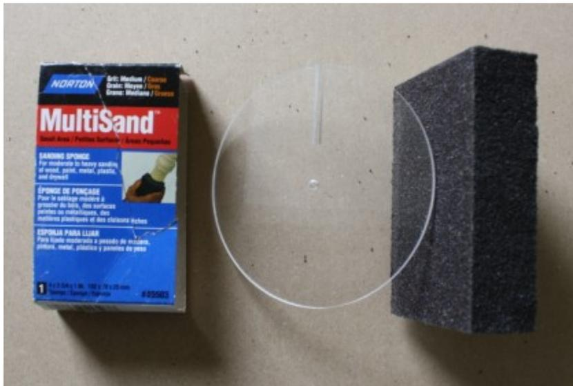
Sand one edge of the disc using medium grit sandpaper, to take the sharp edge off. This will prevent slicing the wire's insulation.
