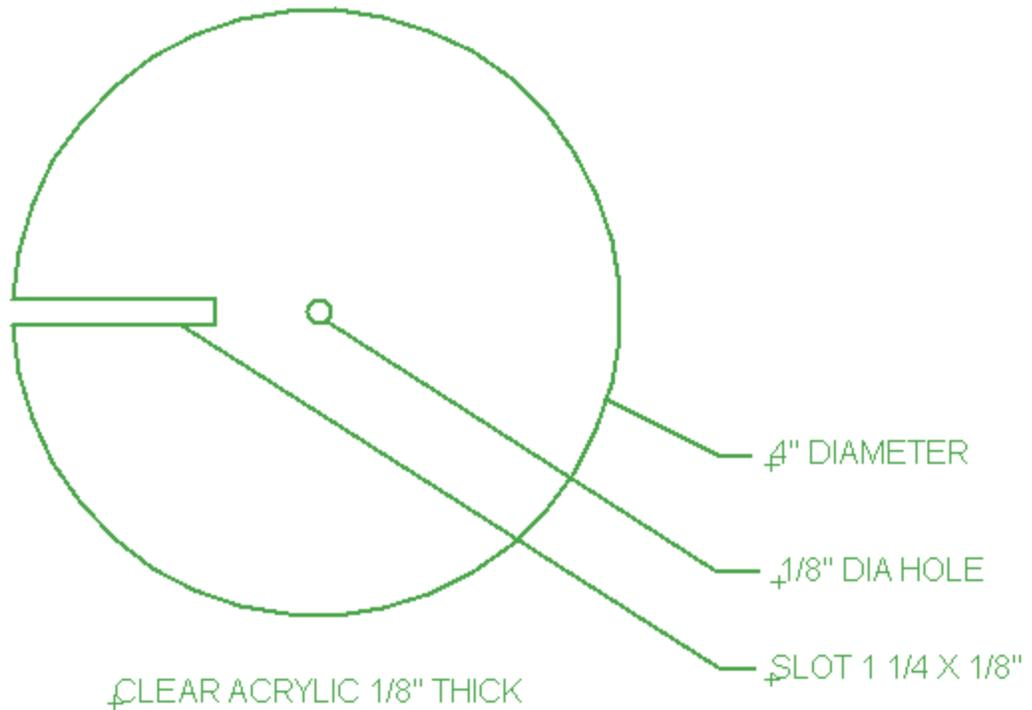
Drill the center hole out to 11/64" diameter.
