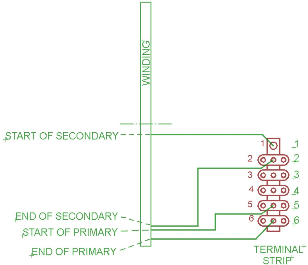
The center end of the Secondary winding goes to the solder lug on the bottom of the board - this is Pin 1.
