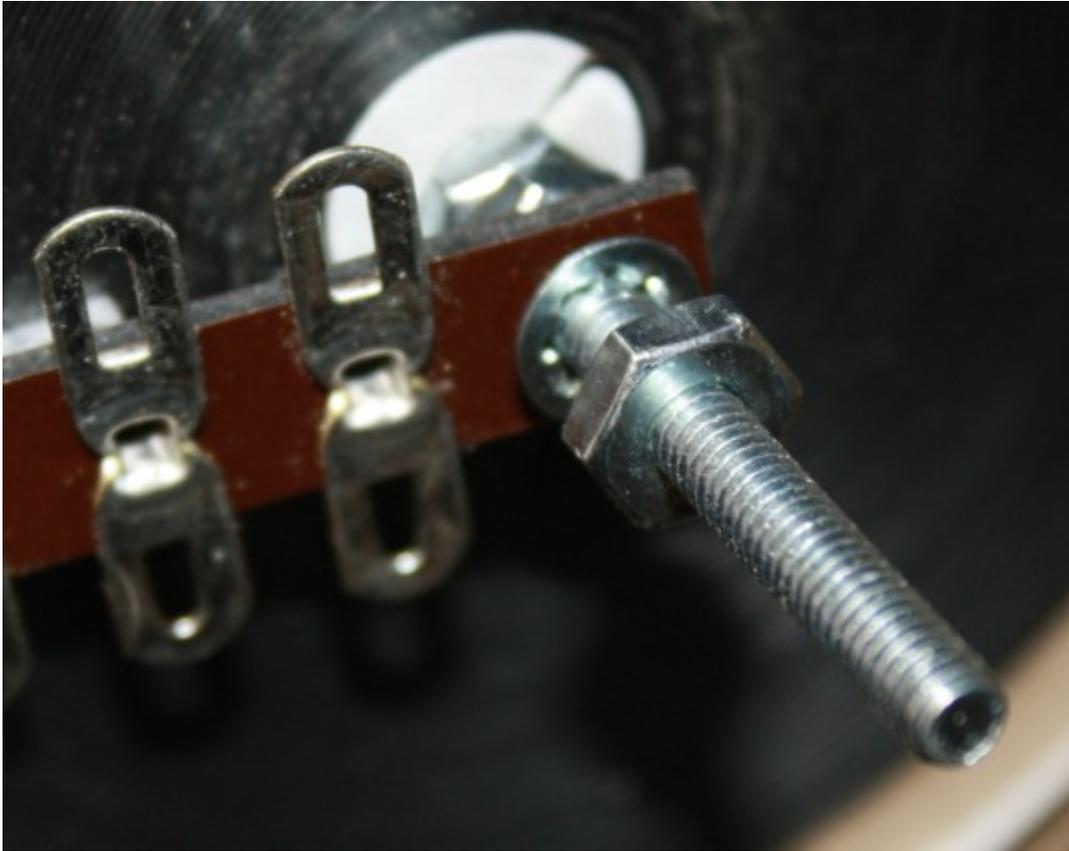
Turn a second 8-32 hex nut onto the screw protruding from the center of the coil that was just wound, and turn it so it sits on top of the first nut. Tighten this nut with pliers. This second nut is just to act as a spacer for the terminal strip, to lift it clear of the disc.
