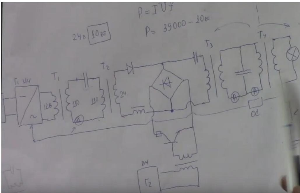
T4 is a phase-shifting transformer (bifilar coil)
