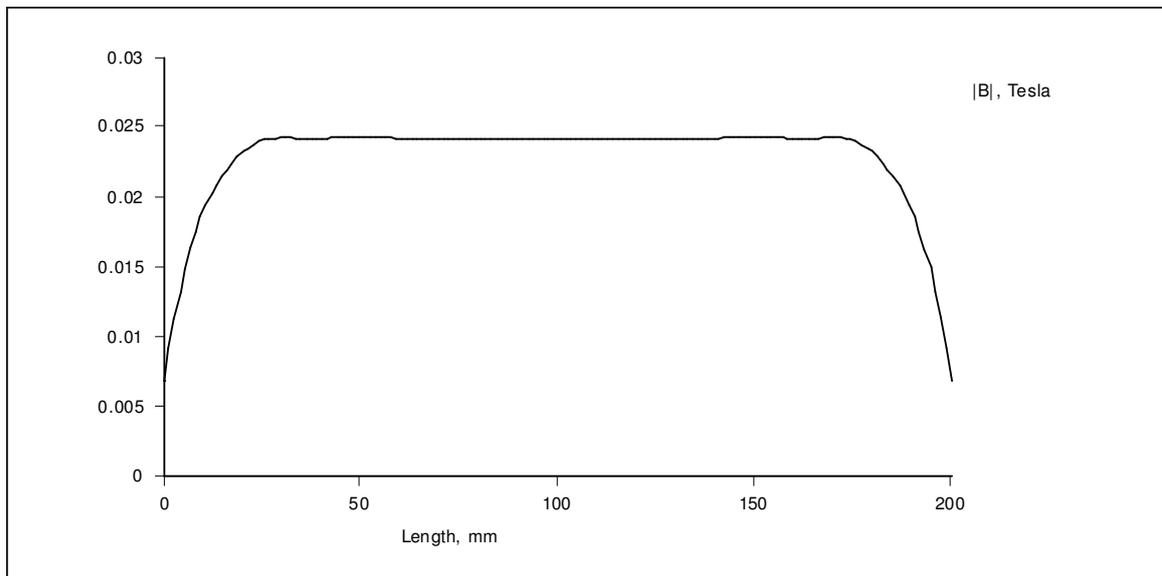
Clearly the use of tapered ampere turns can create uniform field over a significant portion of the core. There is no point in proceeding further with this exercise because FEMM is a 2D model and is showing the field, not within a rod, but within an infinitely long slab. A 3D simulator should enable an optimum coil design to be reached for the cylindrical core.
