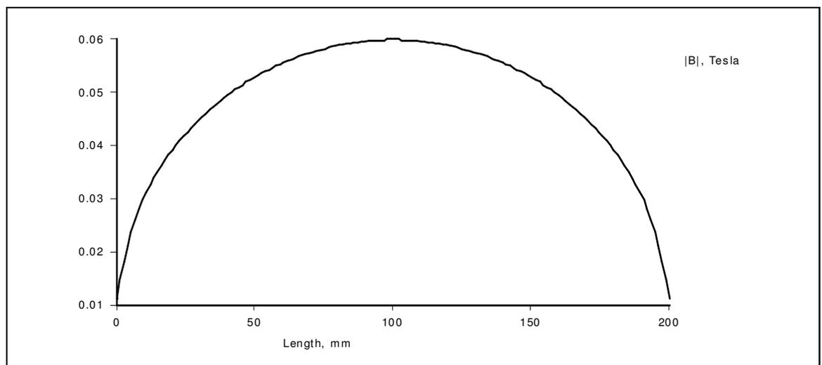
Clearly the field is highly non-uniform over the whole core. The next figure shows seven coils with tapering currents.
