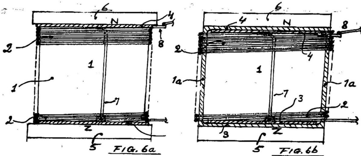
Figures 6a and 6b show MPC's respectively with a primary permanent magnetic field passing through an electron conductor or passing through a plasma.
