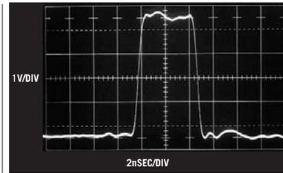
**Figure 3** The 5-nsec-wide output with  $R=390\Omega$  is clean with well-defined transitions. Post-transition aberrations are within 8% and derive from  $G_1$  bond-wire inductance and an imperfect coaxial probe path.
