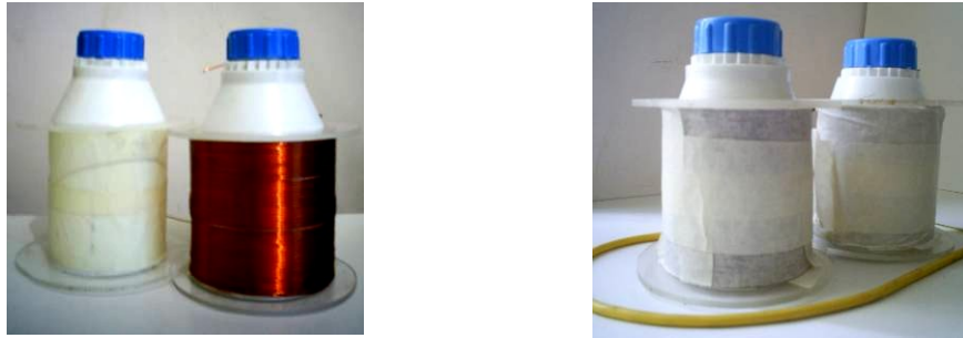
Figure 2: Partially completed sensor at right and completed sensor at left.
