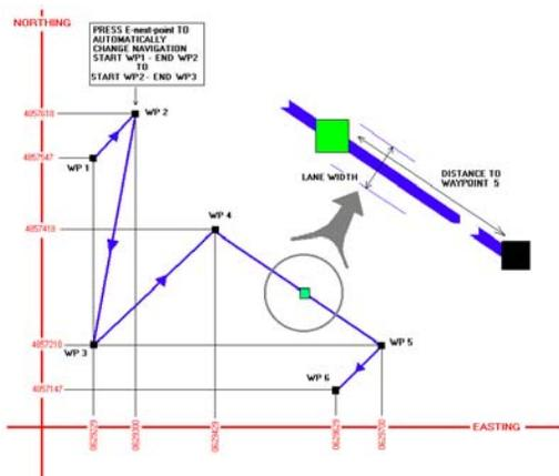
The main benefits lie in survey efficiency and tight survey control for as accurate positioning as possible. You also have the ability to perform surveys along lines that are non-parallel - a useful capability for environmental-type or non-standard, roving surveys.
