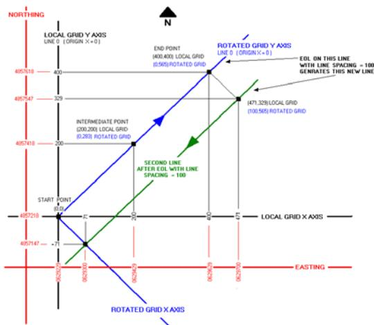
The system then automatically generates a survey grid of 500 lines. You can use as many or as few lines as required to complete your survey.
