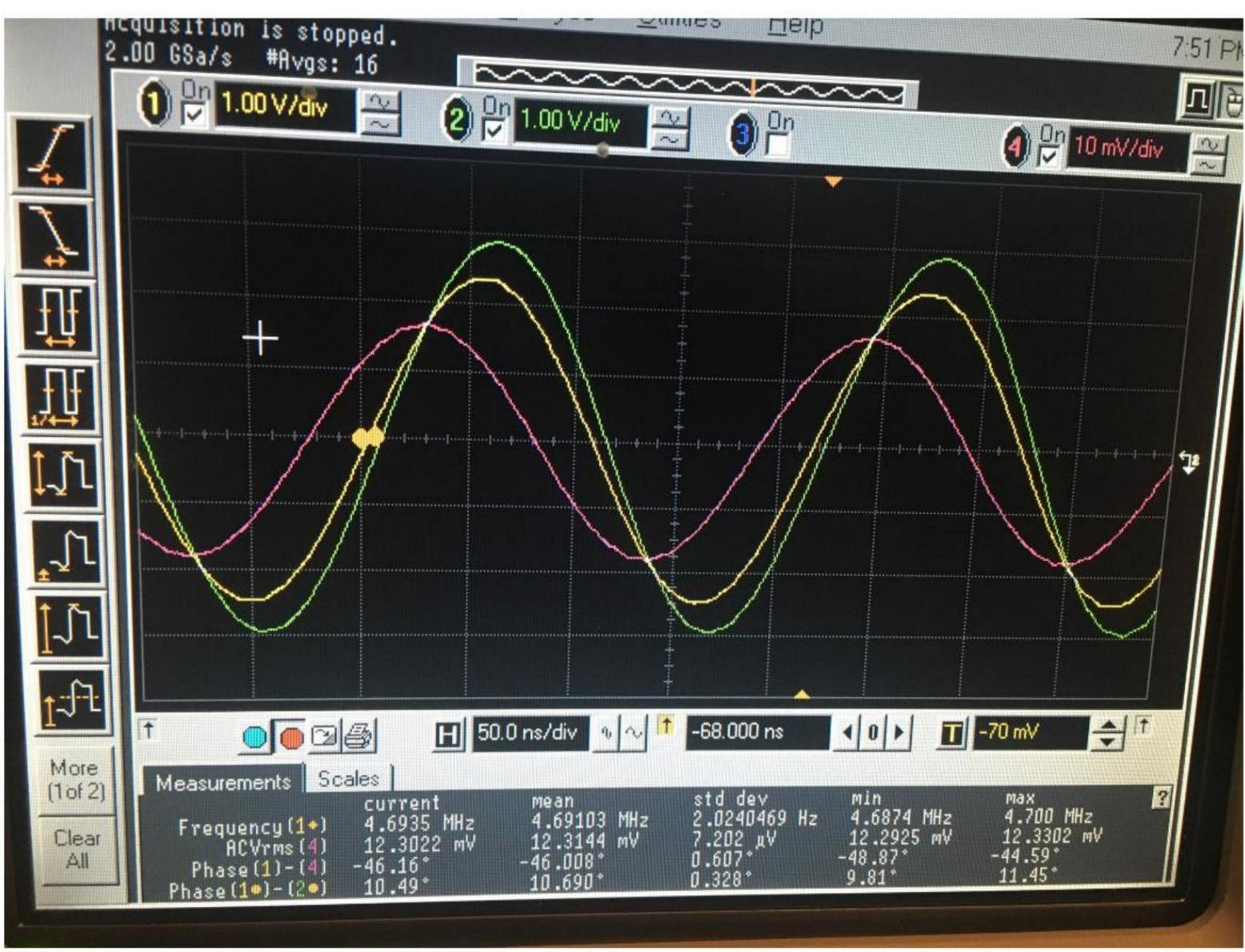
Phase Test 1A.2 - Both A and C are driven at Resonance Test 1A Resonant Frequency.
