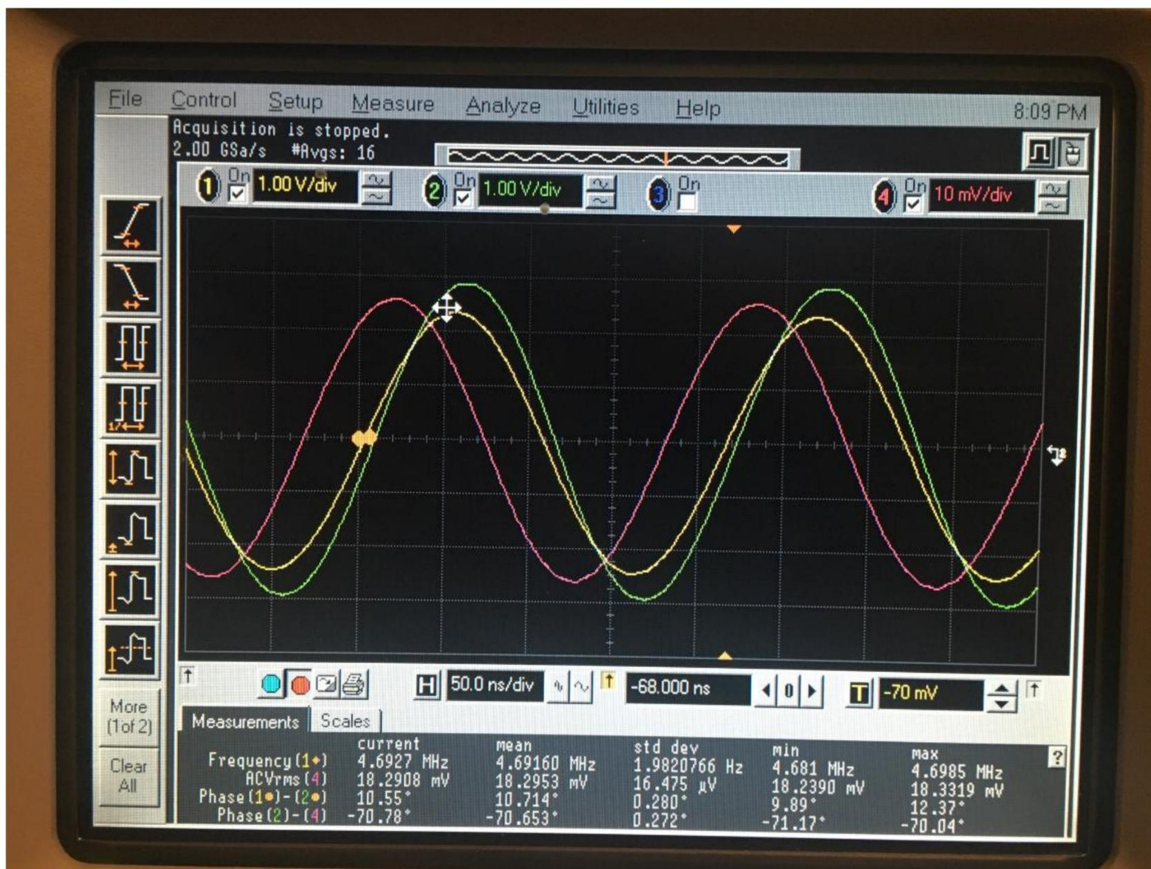
Phase Test 1C.1 - Both A and C are driven at Resonance Test 1C Resonant Frequency.
