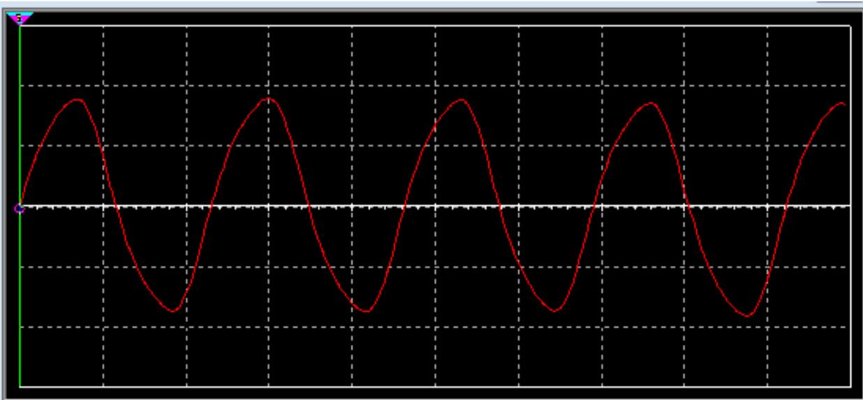
As you can see, in order for us to have a nice sine wave output a 4<sup>th</sup> order filter was necessary.
