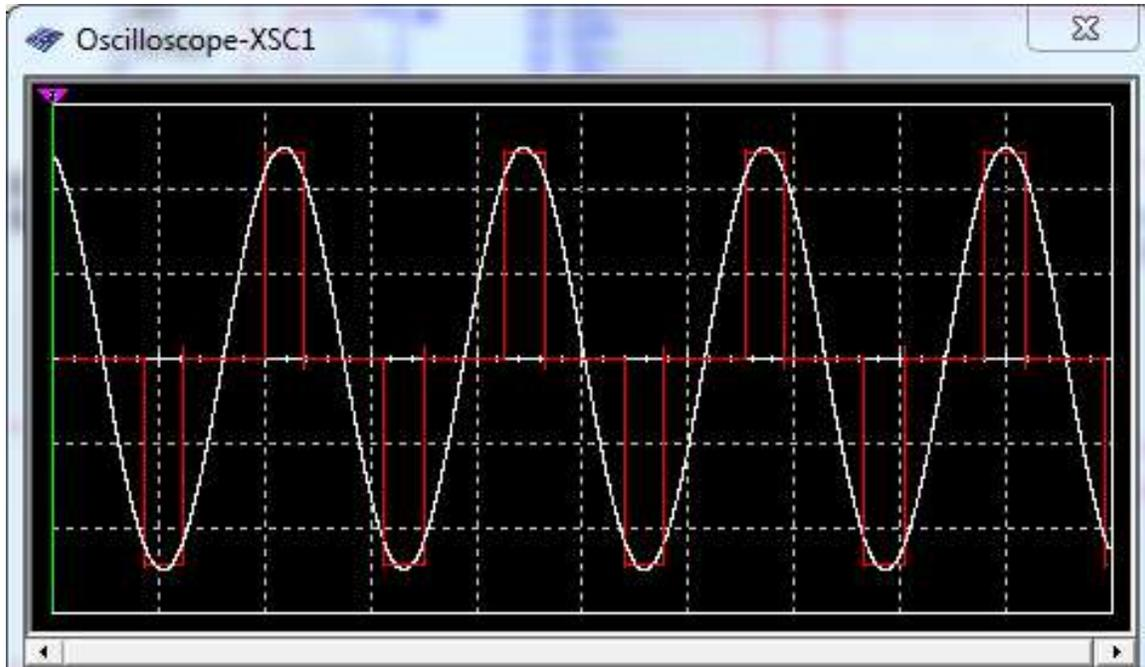
The next stage of our design consisted of the filter stage, where we used a 4<sup>th</sup> order passive filter. The output waveforms shown below will represent what the wave looks like after each stage of the filter.
