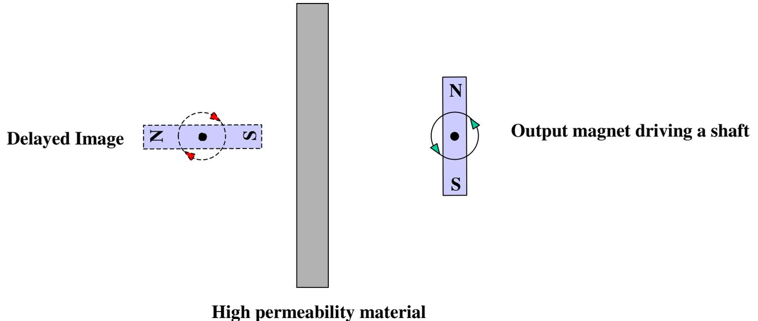
*This is exactly the right orientation for the output magnet to receive a driving torque.* So it seems all we need to achieve self-running is to rotate a magnet close to a sheet of highly permeable material then speed it up until it takes off by itself. Of course life is not that easy, it requires rotation speeds that are too high to be practical. But the principle holds, magnetic delay is a route to overunity.
