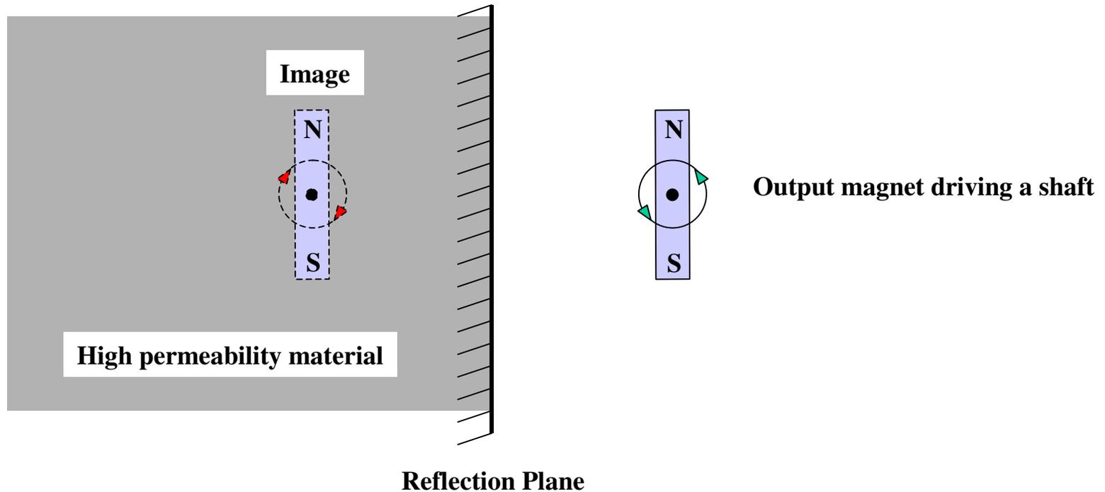
The interesting thing here is that the image rotates on the opposite direction, which is exactly what we want. The downside is that the image does not have the correct orientation.
