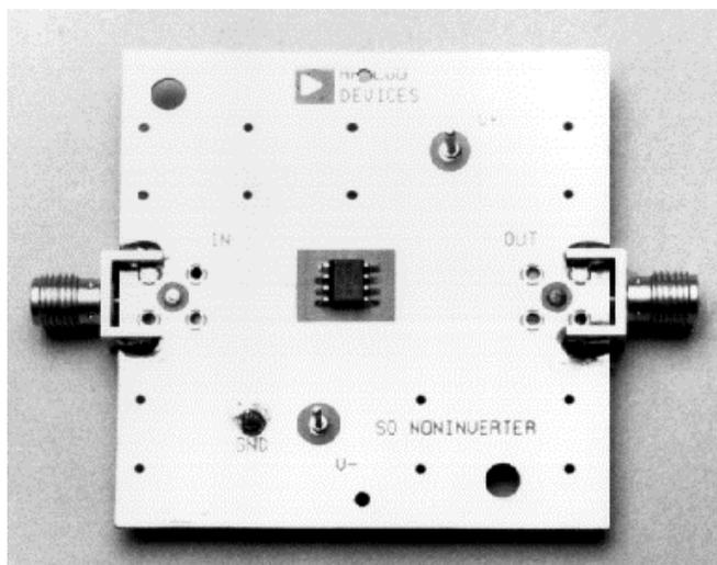
**Figure 13: The AD8001 Evaluation Board Uses a Large Area Ground Plane as well as Minimal Parasitic Capacitance (Top View)**
