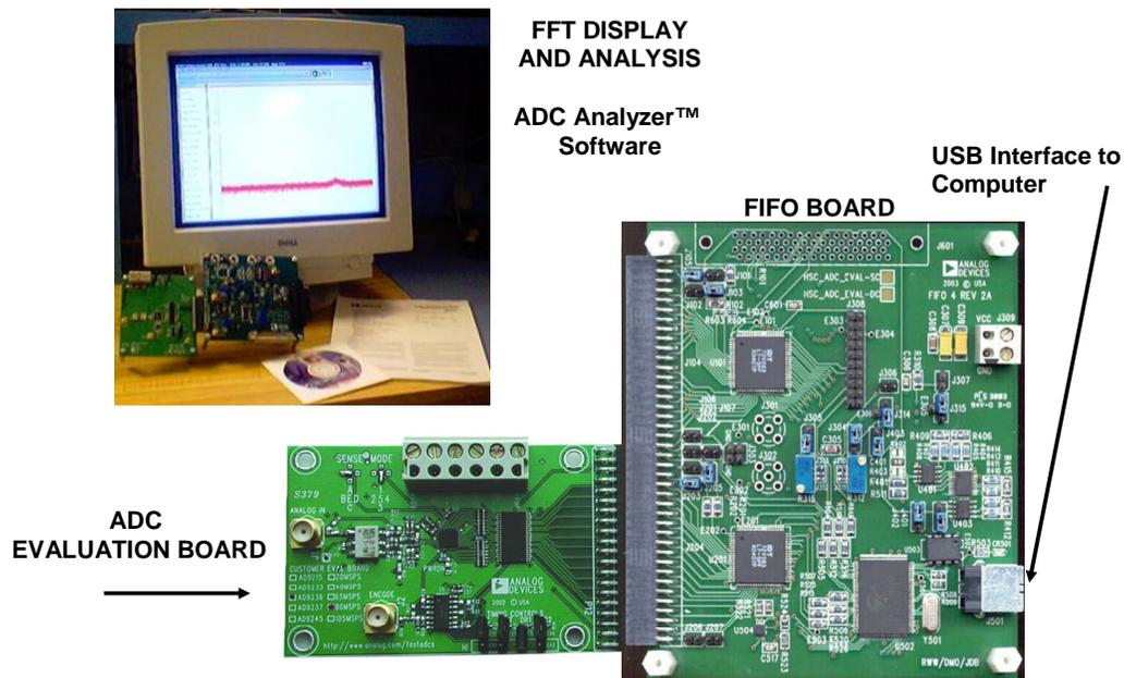
**Figure 14: Analog Devices' High Speed ADC Data Capture Evaluation Kit**
