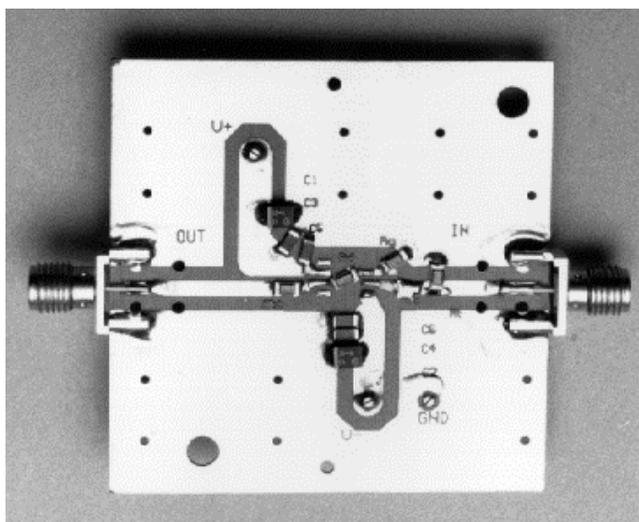
**Figure 12: A High Speed Op Amp Such as the AD8001 Requires a Dedicated Evaluation Board With Suitable Ground Planes and Decoupling (Bottom View)**
