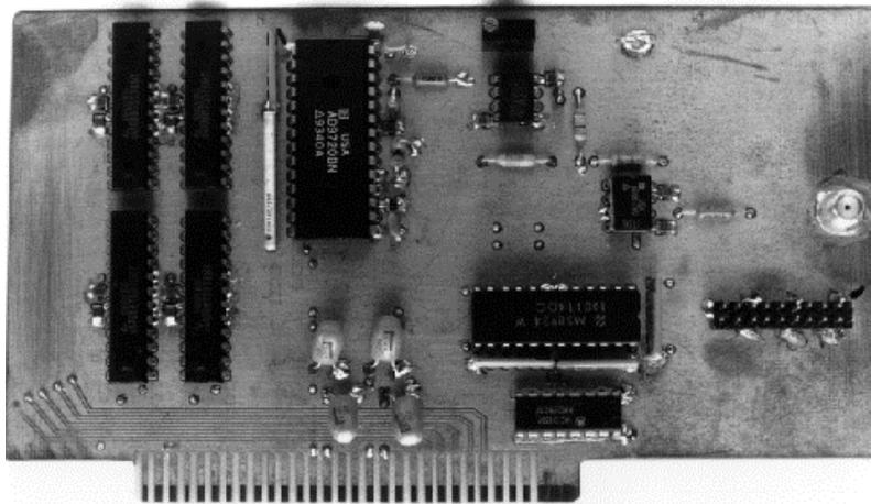
**Figure 4: A Milled Circuit Construction Prototype Board (Top View)**
