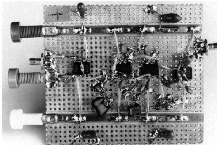
**Figure 3: "A Deadbug" Prototype Using 0.1" Pre-Drilled Single-Sided, Copper-Clad Printed Board Material**
