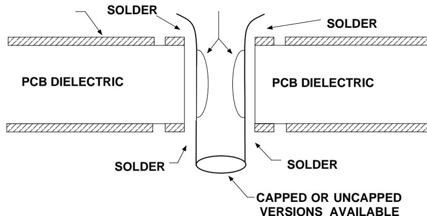
**Figure 6: When Necessary, Use Pin Sockets for Minimal Parasitic Effects**
