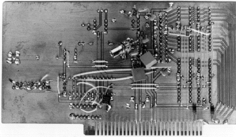
**Figure 5: A Milled Circuit Construction Prototype Board (Bottom View)**
