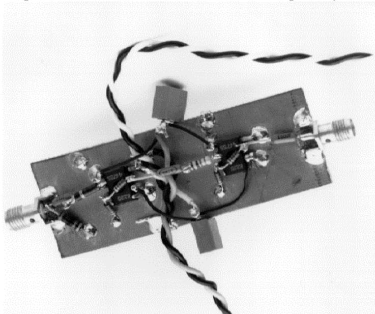
**Figure 2: A "Deadbug" Analog Breadboard**
