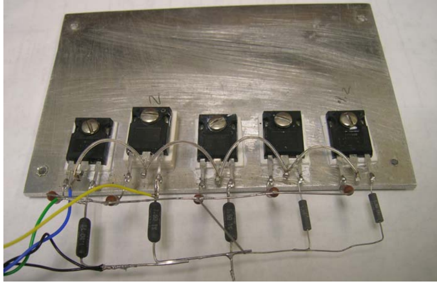
Figure 3. Experimental setup of 5 parallel IRFG50 MOSFETs to demonstrate current hogging phenomenon.
