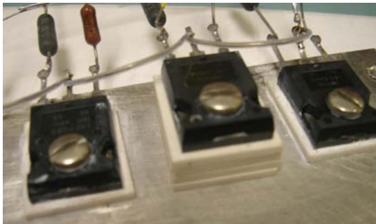
Figure 4. Extra ceramic insulators added to one transistor of Figure 3 to increase its junction to heat sink thermal resistivity.
