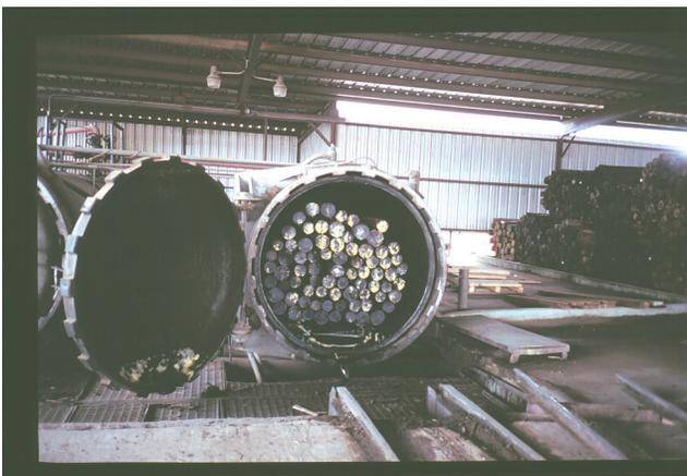
**Figure 3. Pressure treatment tank (Courtesy of Julian Lumber Treatment Company)**
