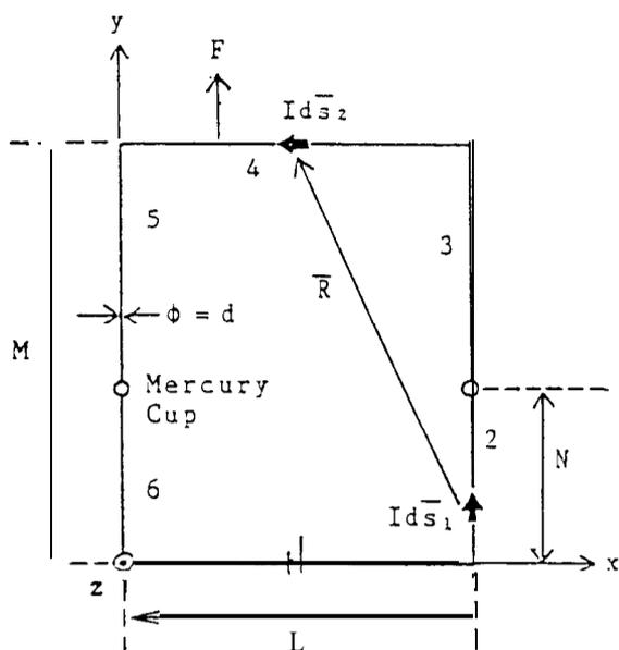
FIG. 4. Diagram of the experiment for the force on Ampere's bridge indicating coordinates, labelling and geometry. The case of straight ends.
