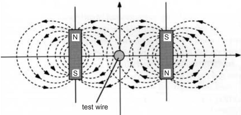
At the point  $x = 0$  and  $y = 0$  for all 'z', the magnetic flux density 'B' is at all times = 0 ! (The field lines of both magnets compensate, which can easily be proven with a Hall probe) The test wire is placed vertically with respect to the x- and y-axis.
