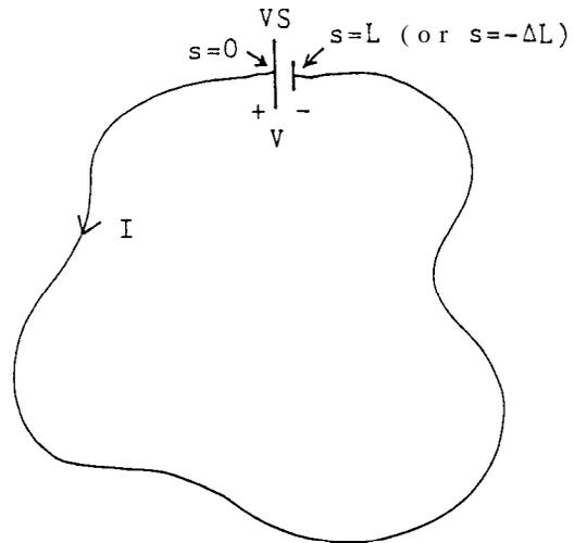
FIG. 3. Model of a closed circuit of arbitrary form, consisting of a capacitor battery and a conductor.
