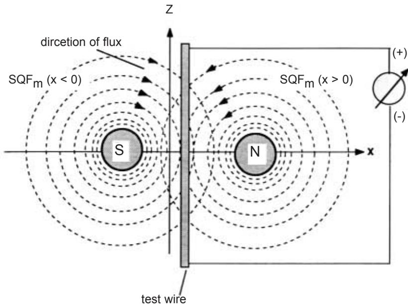
At the place  $x = 0$  and for all 'y' and all 'z' at any time the sum of  $SQF_m (x < 0)$  plus  $SQF_m (x > 0)$  is greater than zero, i.e. the flows are added. These flows (fluxes) push the free charge carriers in the test wire down (-z).
