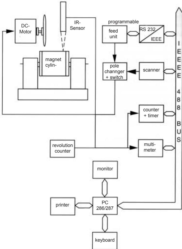
Fig. 19 Electrical-Mechanical Block Diagram of Test Set-Up
