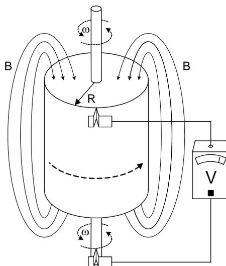
The wheel is consisted of a circular permanent magnet rotating over its axe of symmetry. We believe that during the rotation, magnetic field arising from permanent magnetic disk is not moving on and thus it induces electric field in the rotating disk itself.
