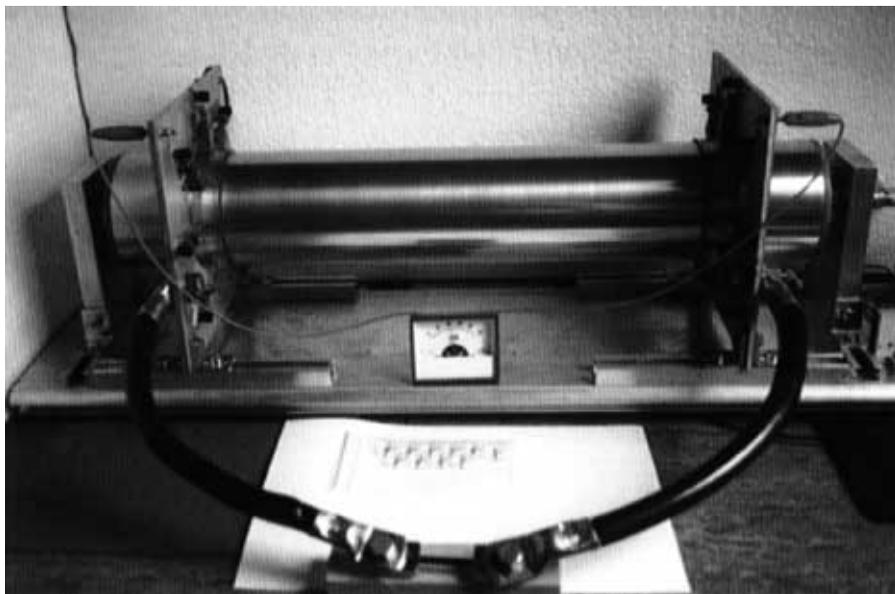
Fig. 2 Detail photo of the C-Generator by Chr. Monstein. Revolutions of 3800 - 4200 r.p.m. depending on the direction of rotation and the use of the same input power for the motor.
