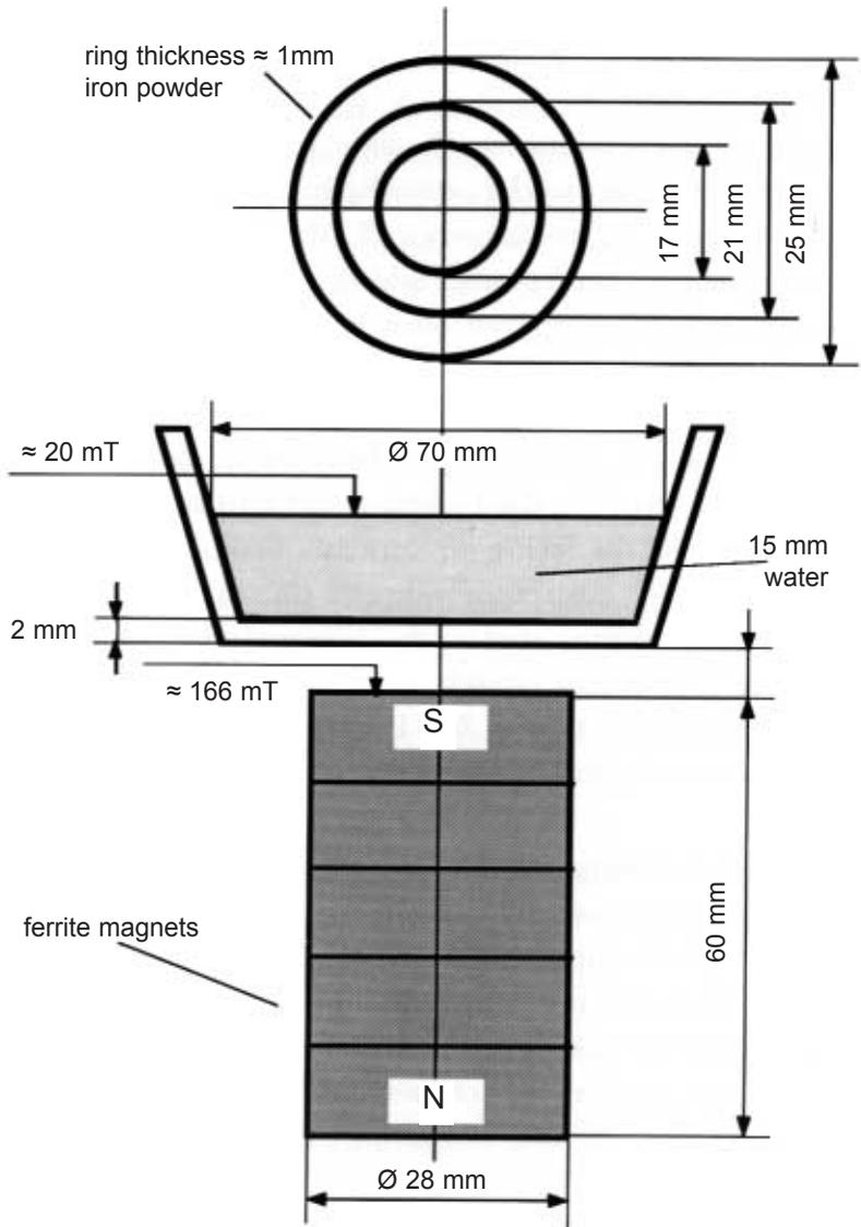
Fig. 13 Ditchev-Experiment Sketch
