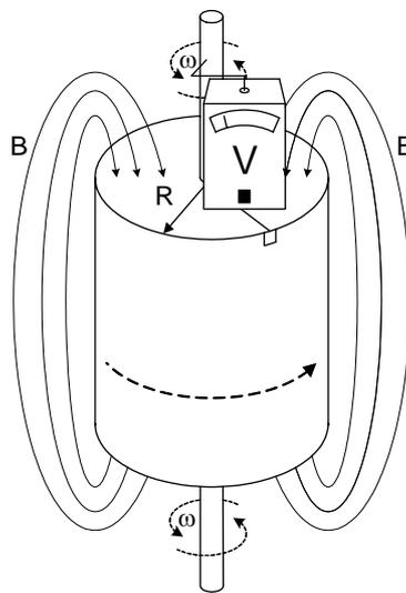
Voltmeter is measuring difference of potential between shaft and border of the spinning disk now. The conductors that lead to voltmeter should be protected from the influence of magnetic field by appropriate shielding.
