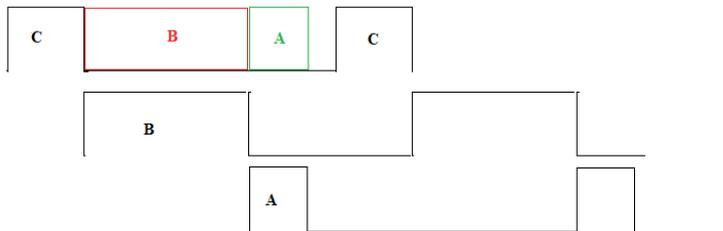
The gap between "A" and "C" is the tuning area for maximum output, increase "C" will move "B" to the right, further increasing "A" will close the gap more. This area is not closed completely and has to be done bit by bit until the maximum kick is obtained, producing the maximum power output.
