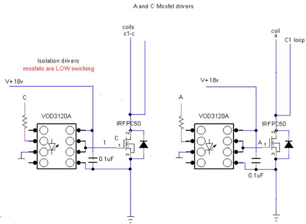
The mosfets shown here are maximum source to drain of 600v and 11amps
