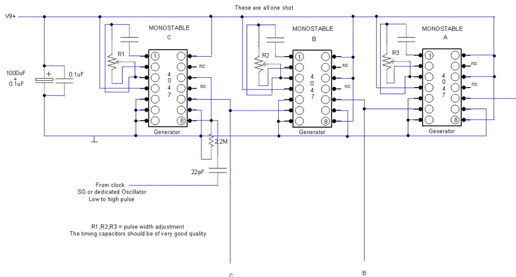
The 22pF cap along with the 2.2M resistor forms a positive going spike to trigger C,
