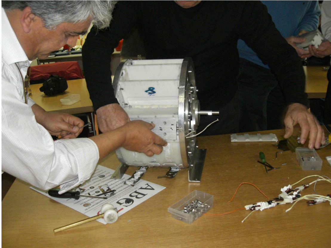
A segment being removed. Note rotor pattern just visible in the next pocket
