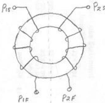
Various connections will be made with the coil wiring. The scope connections will always be CH1(yel) to P1s, CH2(blu) to P2s, CH3(pnk) to output, CH4(grn) input current to P1s, and Math is CH1 x CH4 or input power in mean watts.
