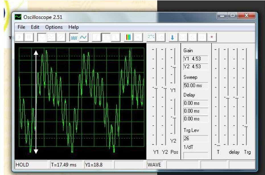
A resonance box is brought close to the speaker until the loudest sound was heard. The signal generator produces the same sound – frequency and amplitude. The Output waveform has a much larger amplitude as indicated by the longer white arrow line. The sound heard is much louder.
