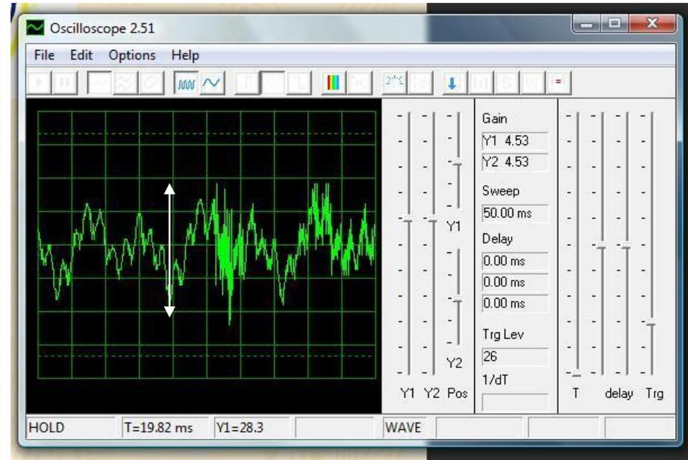
Constant Sound is now produced by the Signal Generator. The signal drives a Toy speaker from the Snap Kit. The sound is picked up by a microphone and The waveform is displayed via the Winscope Program available also from the Snap Kit. Please compare this with the next slide. White arrow shows the peak-to-peak value.
