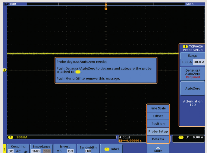
Figure 8. Degauss warning indicator alert from a TekVPI current probe.
