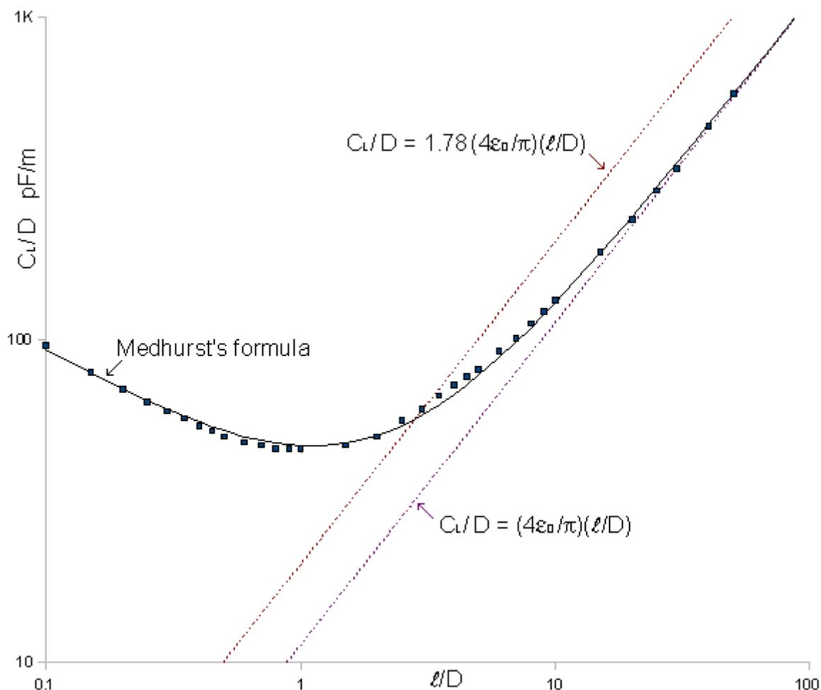
The comparison is given in the graph above, with Medhurst's adjusted data superimposed (spreadsheet: **Medhurst.ods**, sheet 2).
