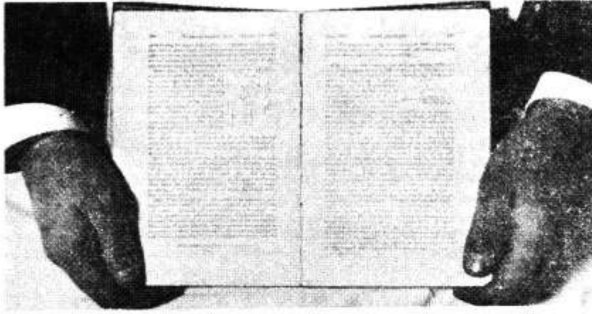
PHOTOGRAPHED BY THE LIGHT OF A SINGLE VACUUM TUBE AT A DISTANCE OF FOUR FEET; EXPOSURE TWO SECONDS.
