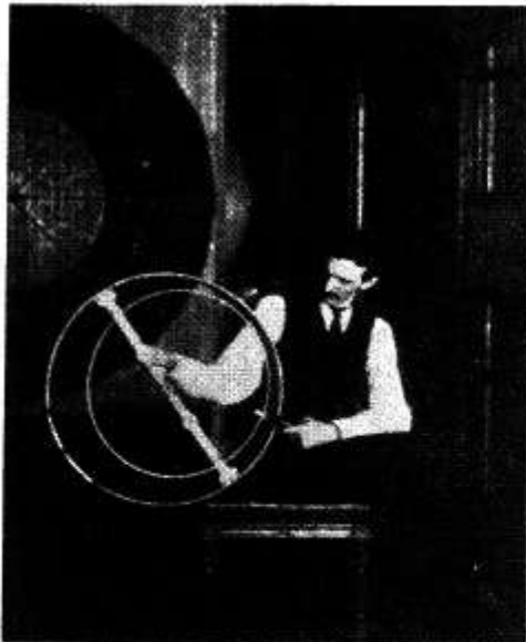
FIG. 7 - EXPERIMENT SHOWING A COIL ENERGIZED BY THE WAVES OF A DISTANT OSCILLATOR AND ADJUSTED TO THE CAPACITY OF THE BODY OF THE OPERATOR, WHO PRESERVES HIMSELF FROM INJURY BY MAINTAINING A POSITION AT THE NODAL POINT, WHERE THE INTENSE VIBRATION IS LITTLE FELT - THE PRESSURE ON THE END OF THE COIL TOWARDS THE READER, WHICH IS ILLUMINATED BY THE POWERFUL STREAMERS, IS NEARLY HALF A MILLION VOLTS.
