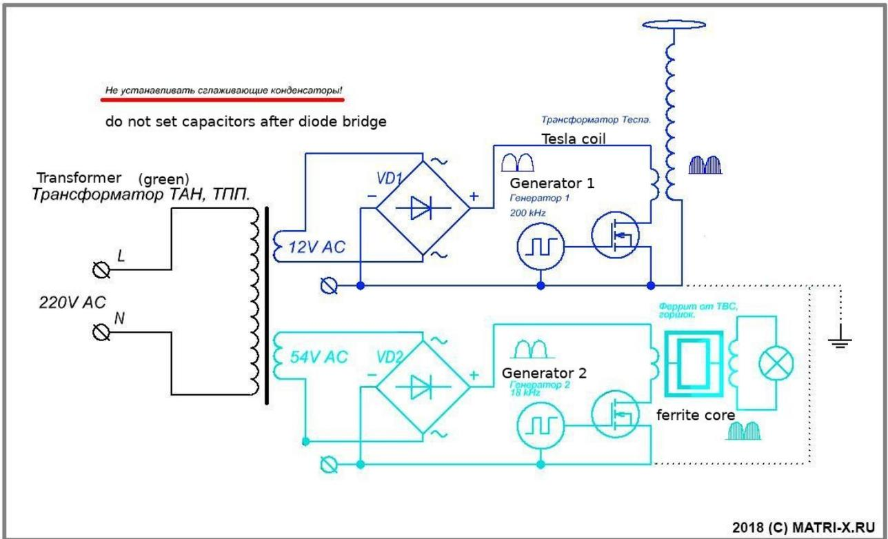
supposingly experiment schematic (generator 2 is push pull in the video)
