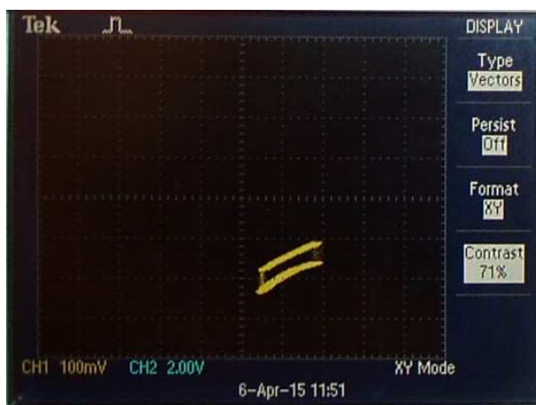
ferrite core with PM, demagnetization on the bottom (now shifted up)
