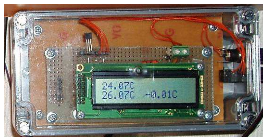
pic. dual temperature sensor in velleman box
