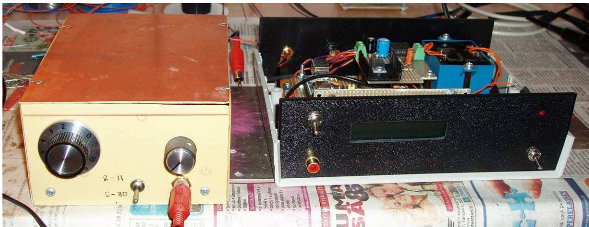
pic. Frequency meter (on the right) with signal source (on the left)
