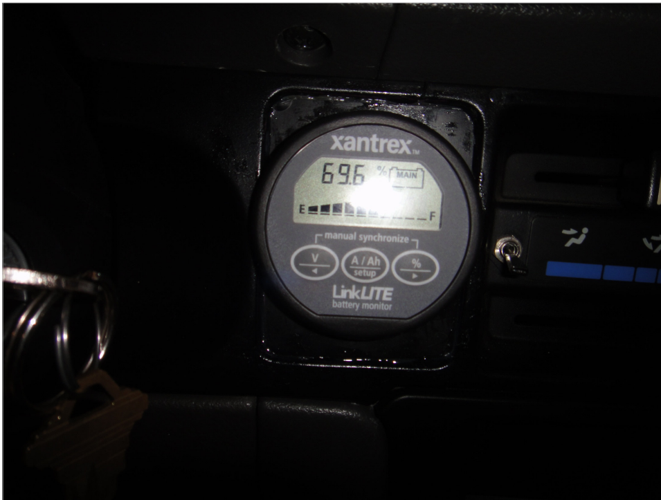
Dashboard gauge inside the Solectria. It gauges the amount of energy remaining in the battery. This 69% value was after driving for about 20 miles with four passengers
