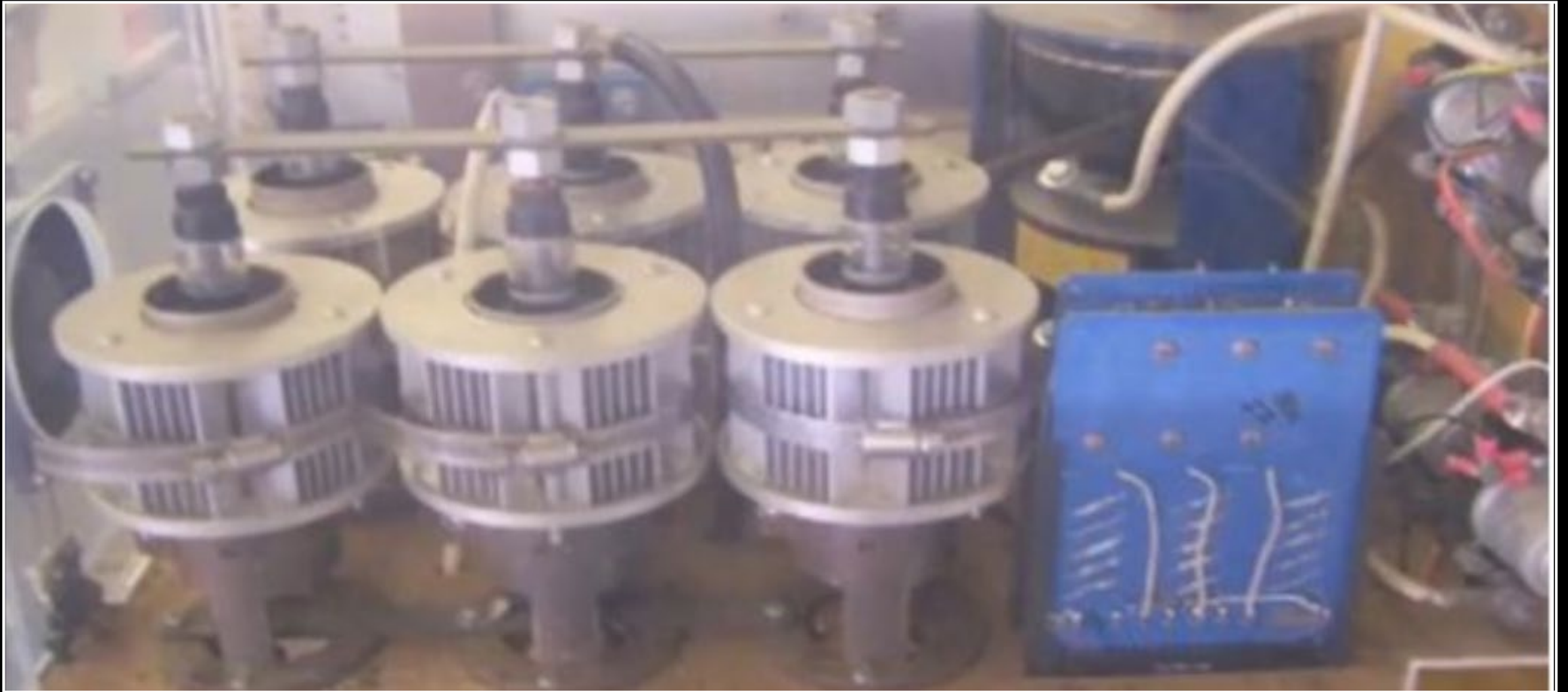
Gold Motor Ignitron Bank - Two Ignitrons per Pole
