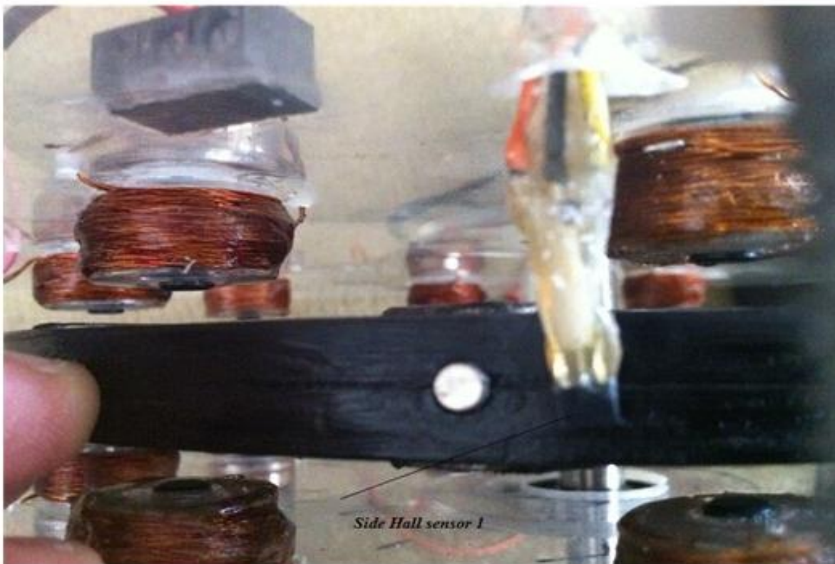
Second hall sensor uses the 8 outer magnets.
