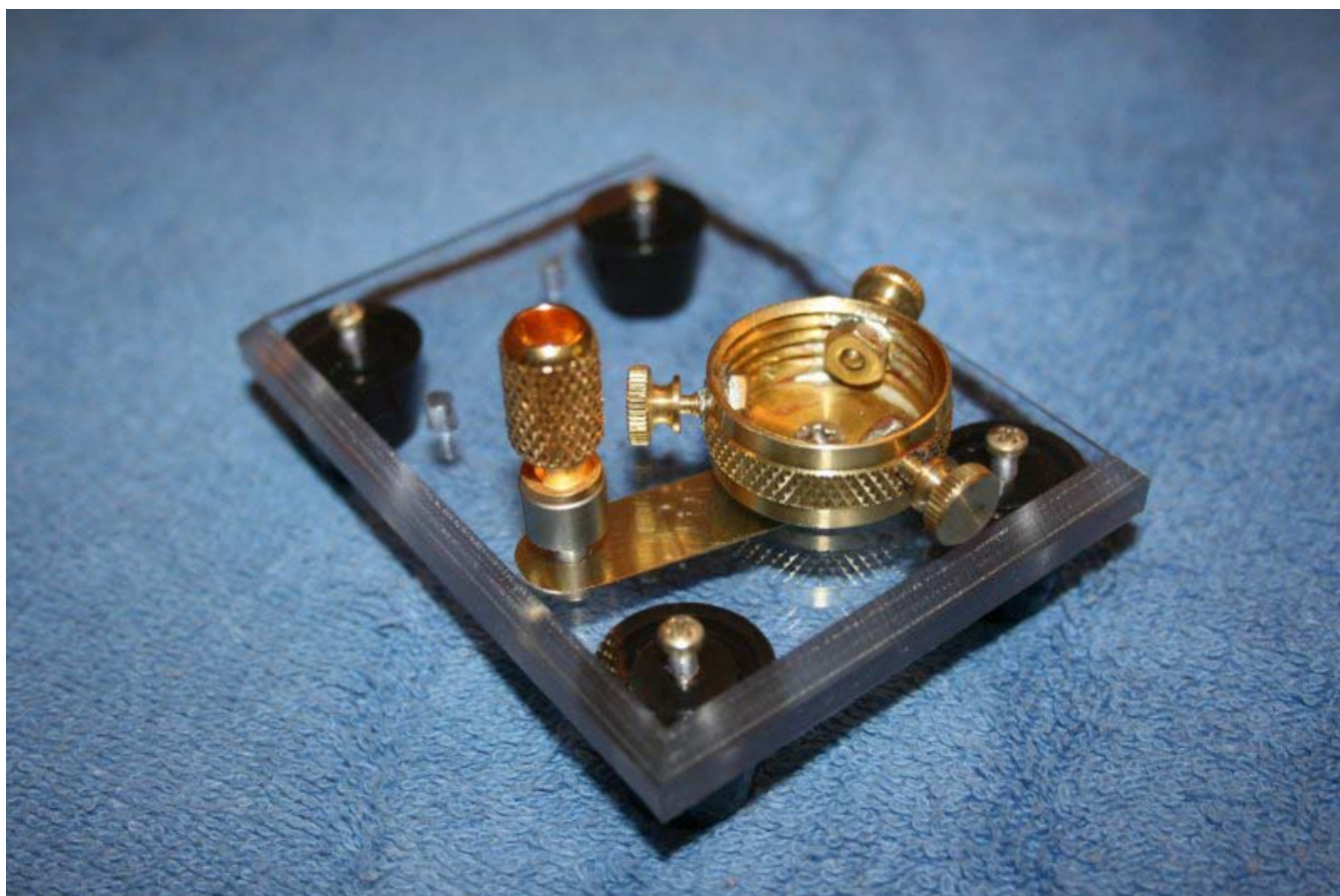
A brass strip makes electrical contact between the binding post and the sample holder
