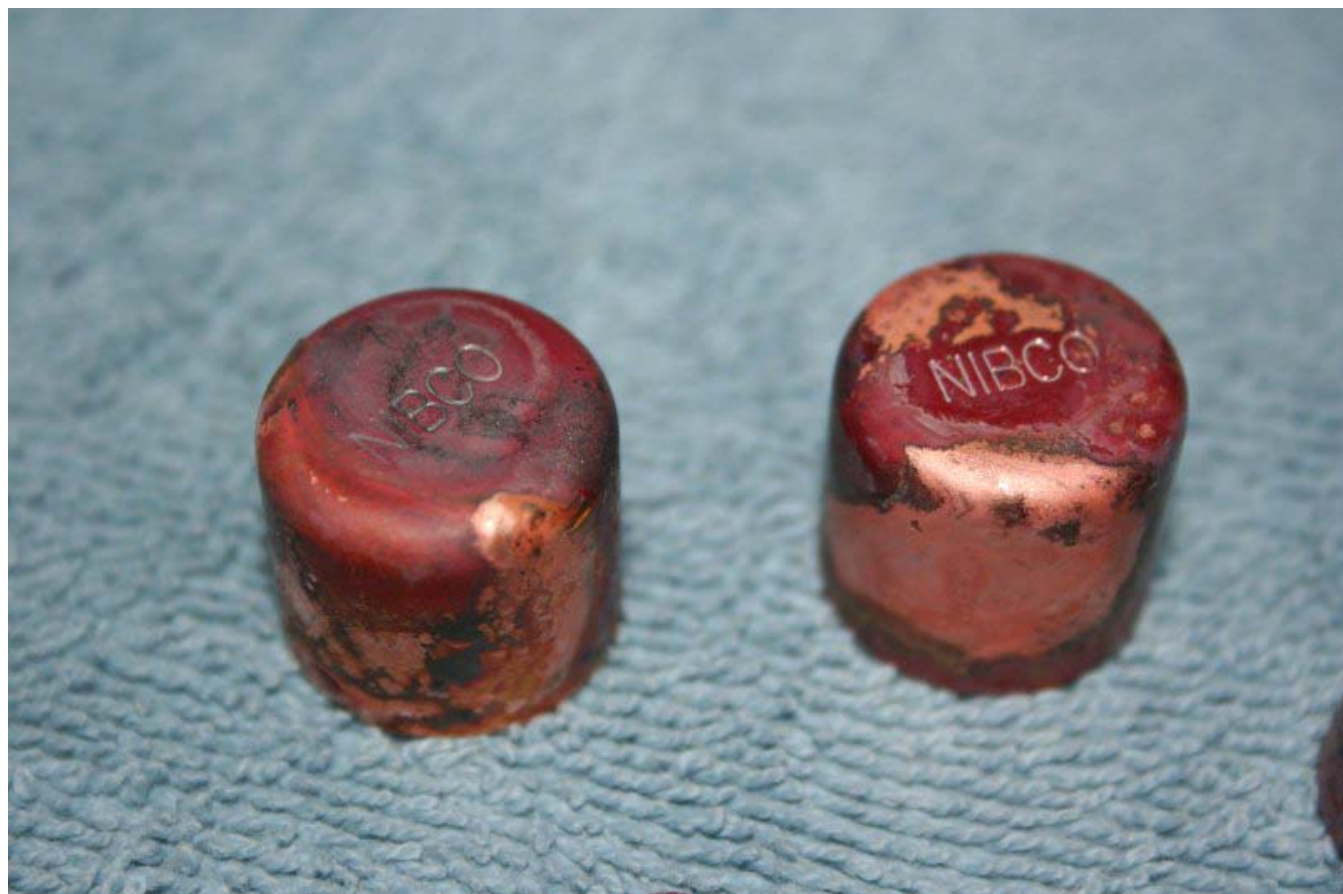
Treated copper pipe caps with cuprous oxide coatings
