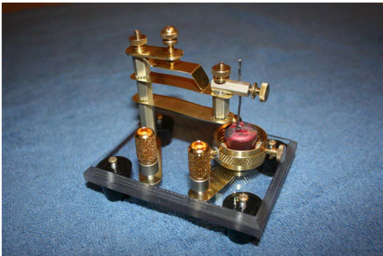
The completed cuprous oxide detector (diode)
