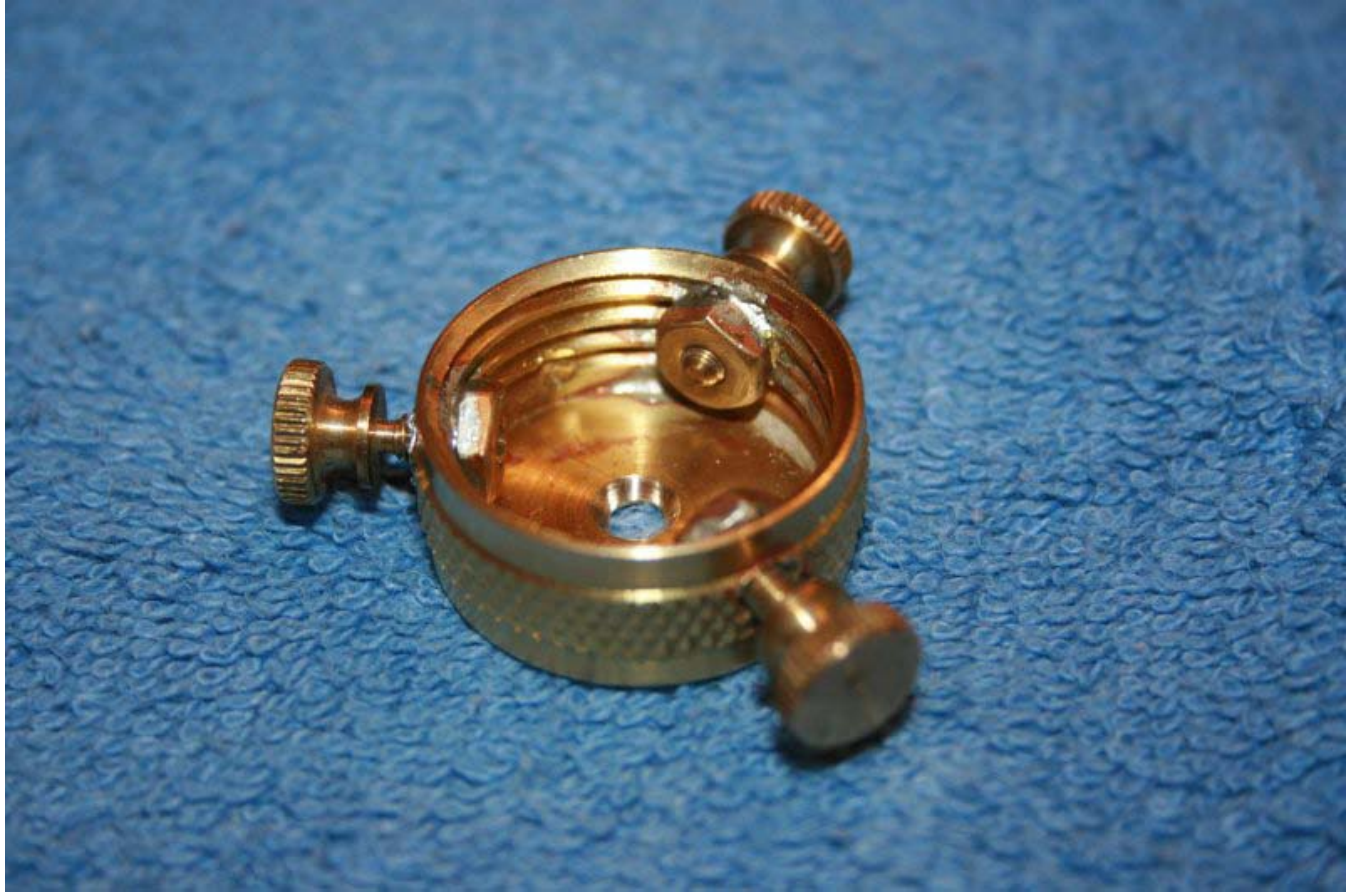
The instrument's "sample holder"
