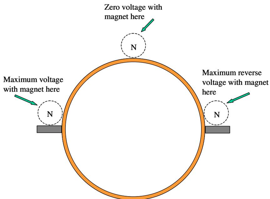
**Figure 4. Initial experiments with different magnet positions**
