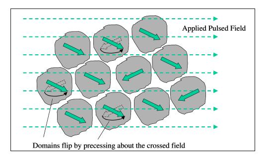
If this theory holds water the precession frequency could be peculiar to the anisotropic highperm material, and may not occur in other materials. The relatively low frequency of Graham's device suggests that the frequency could be associated with the stress and strain characteristics of the material, the torsional stress on each grain changes direction when the dipole flips.
