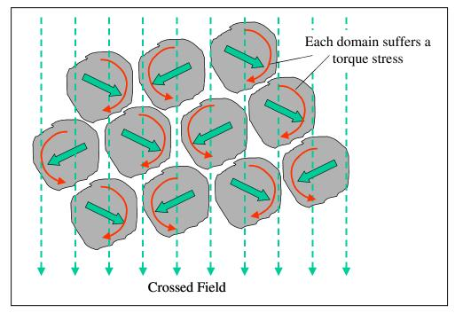
The application of a high magnitude cross-field results in only a small sideways magnetization, the material exhibits low permeability in that crossed direction. It may now be conjectured that the application of a pulsed field along the core axis that will cause some of
